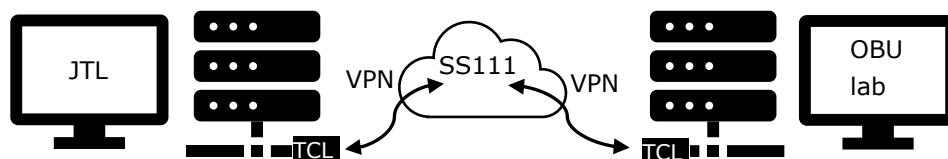
Figure 2: Connection facilities for remote JTL testing
